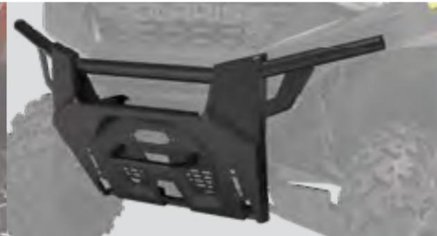
1 3/4" DIAMETER STEEL TUBE CONSTRUCTION
