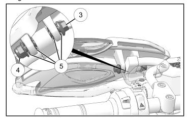
8. Put *hand guard* in desired position. Counter-hold nut (4) and tighten bolt (3) until fully seated.
