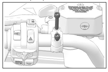
6. Install left-hand hand guard mount ② with two screws ⑥. Torque to specification.
