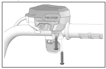
2. Install right-hand hand guard mount ① to bottom of handlebar with two screws ⑦. Tighten until fully seated.
